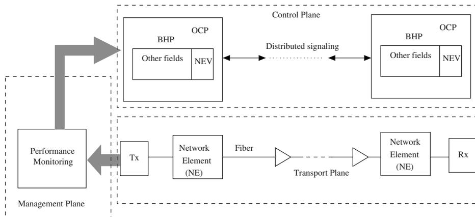
Fig. 1. Structure of the control plane for the distributed signaling.
