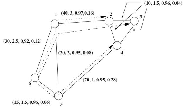
Fig. 4. Network example used to explain the proposed algorithm. The weights on the links indicate distance, noise factor, reliability, and propagation delay.
