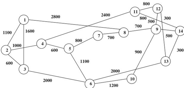
Fig. 5. Network topology of NSF network, consisting of 14 nodes and 21 bidirectional fiber links.
