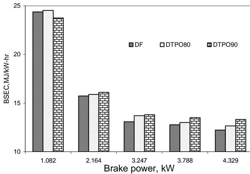
**Figure 5 Variation of BSEC with brake power**
