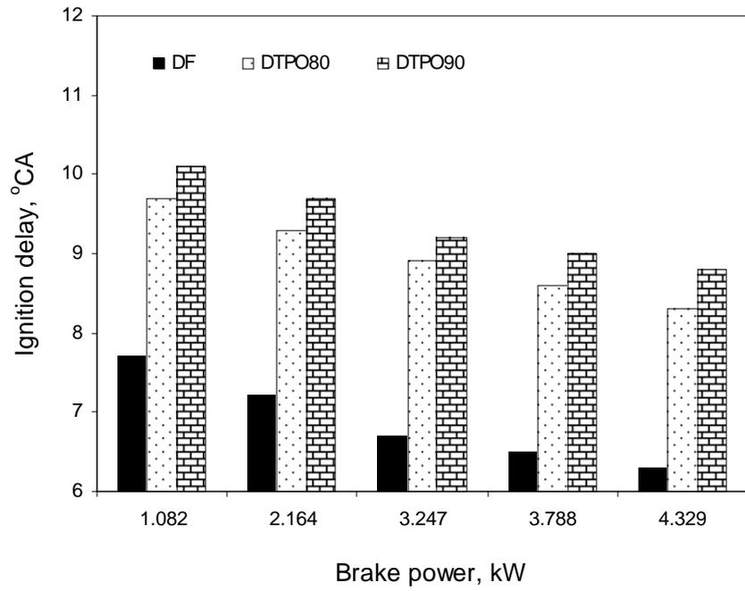
**Figure 12 Variation of ignition delay with brake power**
