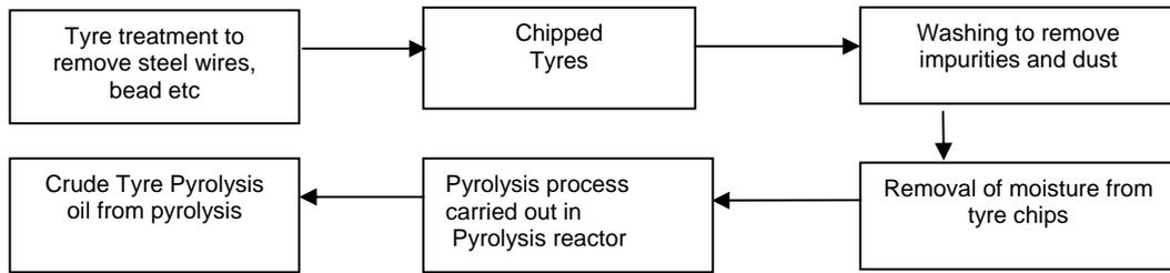
**Figure 1 Pyrolysis process of waste automobile tyres**
