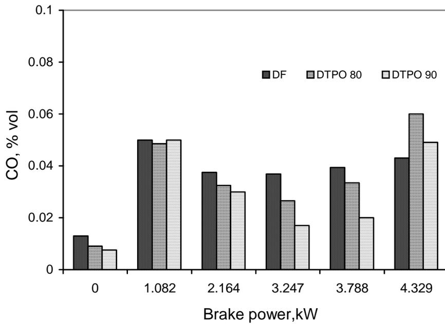
**Figure 9 Variation of CO emission with brake power**
