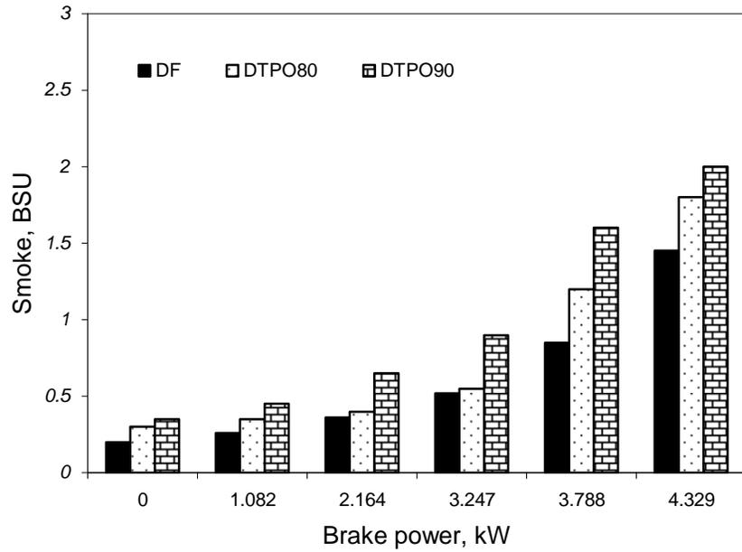
**Figure 10 Variation of Smoke with brake power**
