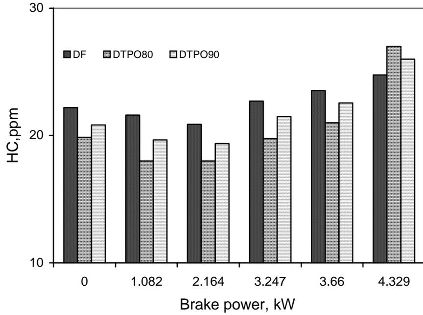
**Figure 8 Variation of Hydrocarbon emission with brake power**
