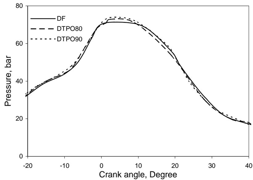
**Figure 11 Variation of pressure with crank angle**
