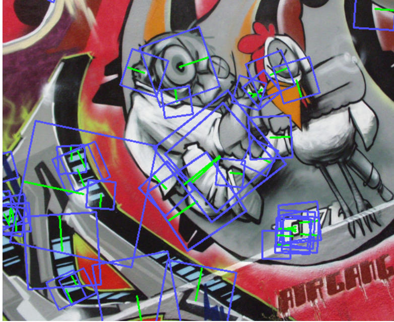
Figure 8: Descriptor Windows. The window size is 20 times the scale of the detected point and is oriented along the dominant direction shown in green.
