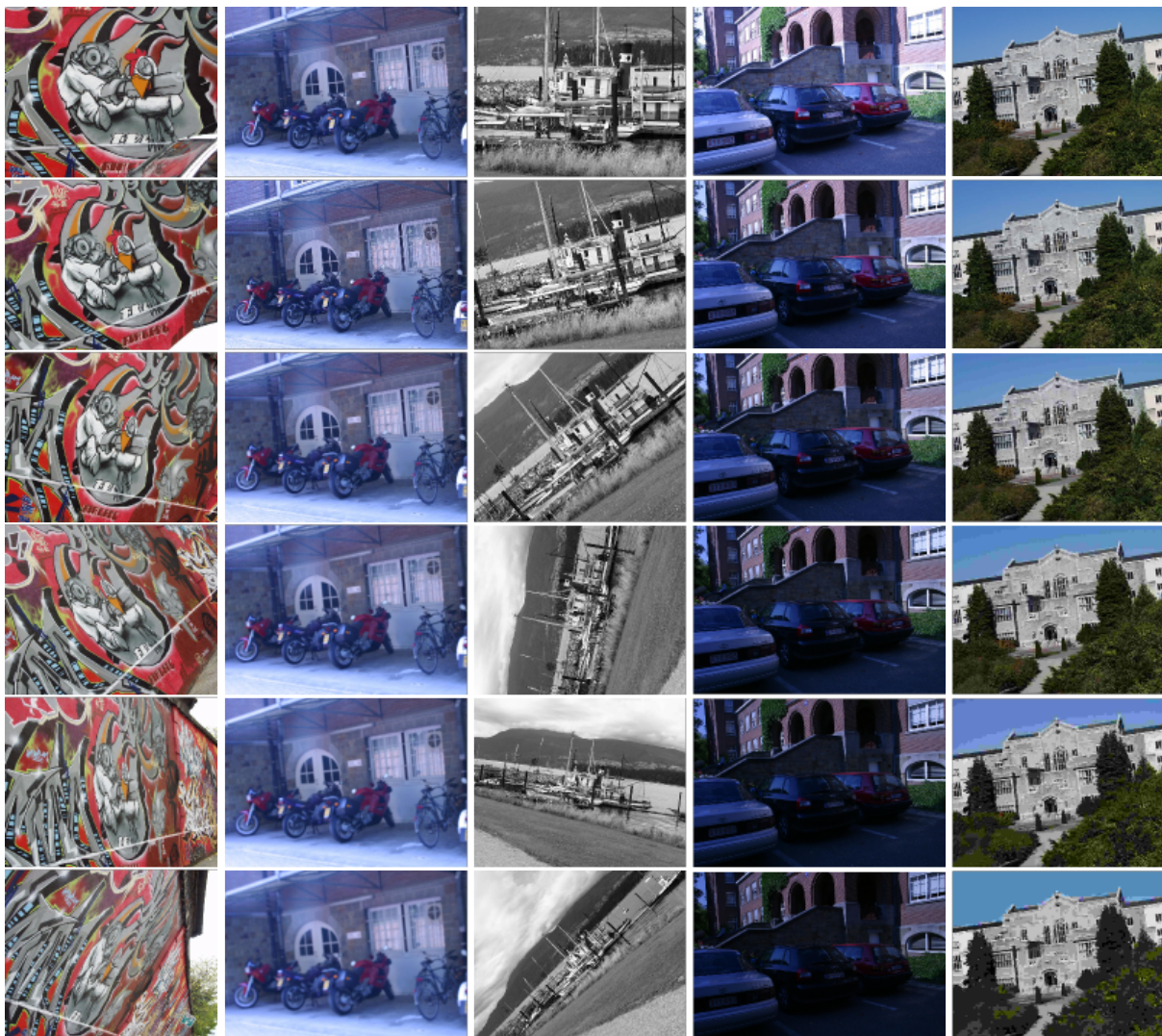
Figure 10: Test Dataset. Columns left to right: Graffiti with viewpoint rotation, Bikes with blur, Boats with optical axis rotation, Leuven with brightness and UBC with JPEG compression.
