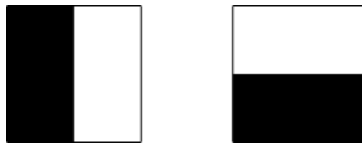
Figure 6: Haar Wavelets. The left filter computes the response in the x -direction and the right the y -direction. Weights are 1 for black regions and -1 for the white. When used with integral images each wavelet requires just six operations to compute.
