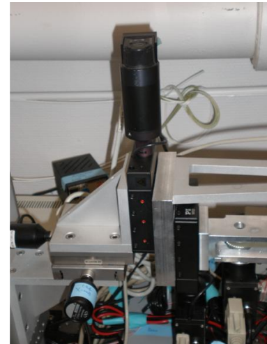
Figure 69: Photograph of the structure for holding the magnets. The structure is linked to two translation stages allowing for displacement in the XY-plane (photograph on the right). Those are in turn connected to a supporting column which is fixed directly on an optical table.
