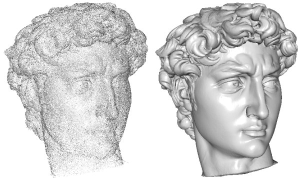
Figure 2: Visualization of the raw data returned by 3D scanners (left) and a surface reconstruction fit to the data (right).
