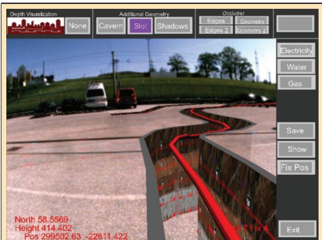
Figure 3. X-ray vision visualization used in the Smart Vidente project to visualize underground water and gas pipes.
