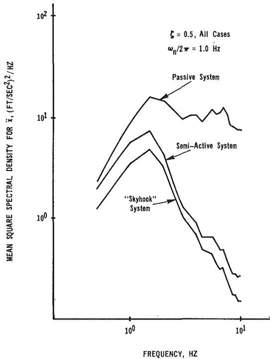
Fig. 9 Typical random input response plot
