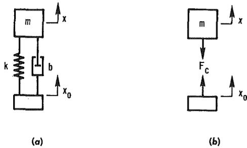
Fig. 1 Isolation of a mass from ground motion: (a) Passive linear isolator and (b) Active isolator: Force  $F$  is supplied by a servomechanism
