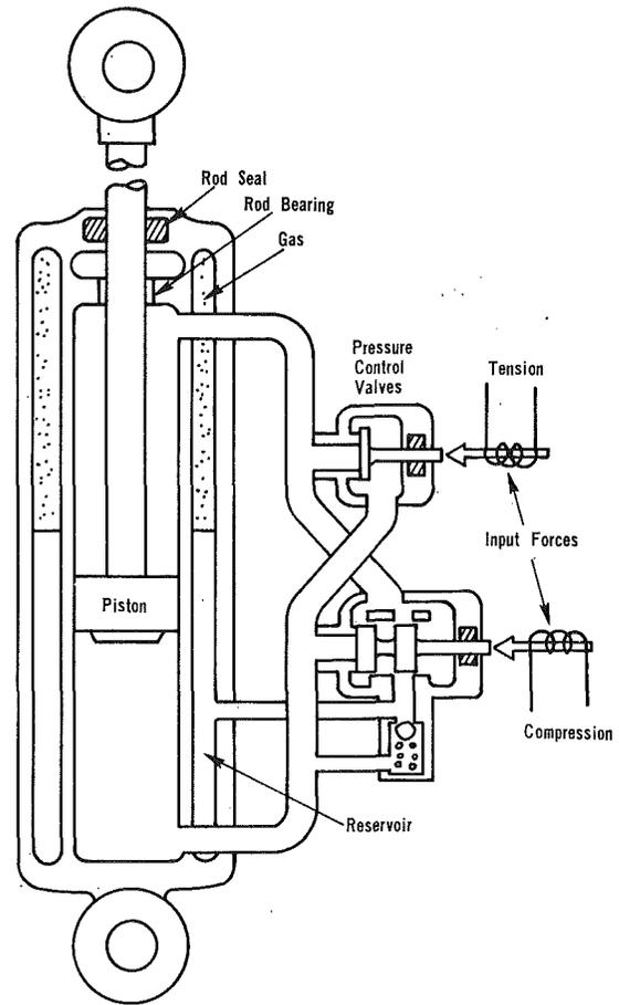
Fig. 10 Electro-hydraulic active damper schematic
