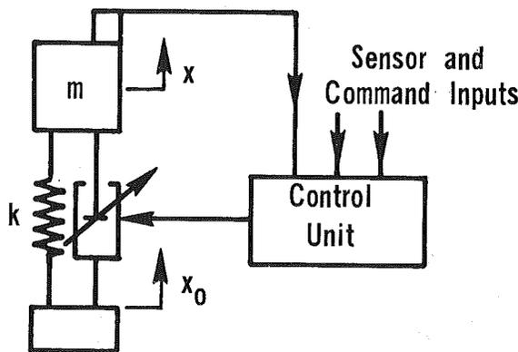
Fig. 4 A semi-active isolator system
