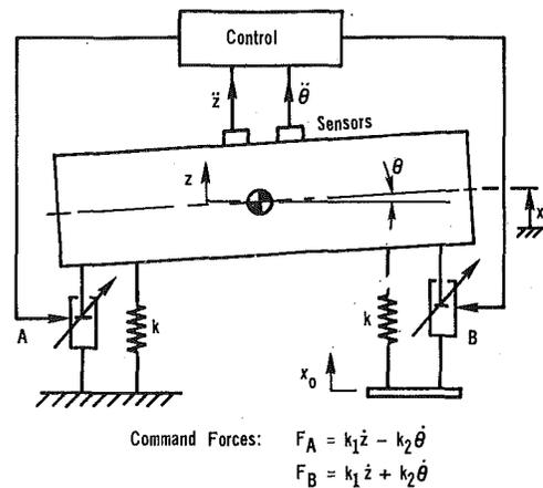
Fig. 12 Semi-active control of two degree-of-freedom system
