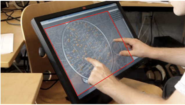
Figure 6: Our user study took place on a commercially available and freely tilttable 22" multitouch screen. The red area marks the portion of the screen we used for the interaction.
