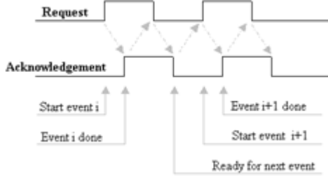
Figure 2: 4-phase Asynchronous Signalling Protocol
