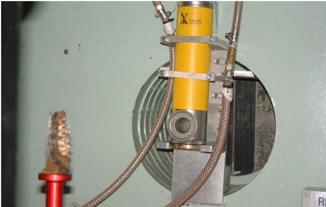
Fig. 6.5 - Set up of the partial mandible of *Theropithecus oswaldi* fixed with putty onto the rotary disk and positioned between the X-ray source (the yellow tube in the picture) and the scintillator screen (not visible here)
