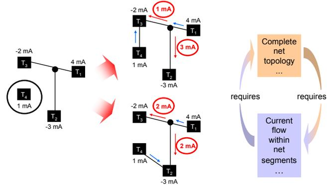
**Figure 12.** Illustration of the cyclic conflict whereby the sequence of all terminals to be connected must be known in order to allow for a current calculation within net segments. At the same time, laying out the sequence of connections requires currents to be known in order to fulfill certain optimization criteria.
