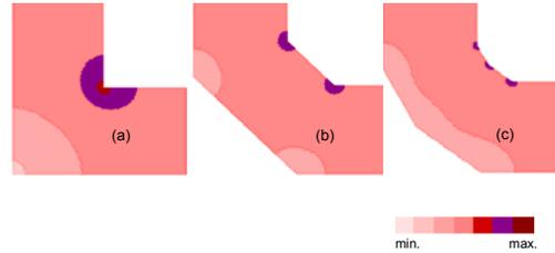
**Figure 8. Current-density visualization of different corner bend angles of (a) 90°, (b) 135°, and (c) 150°.**
