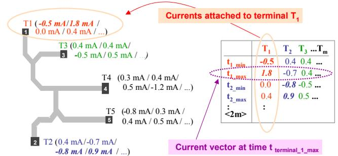
**Figure 10. An illustration of the first approach utilizing current vectors. Current values assigned to terminals are their respective minimum and maximum values (shown in *italic*) and the current values at the other terminals’ minimum and maximum points of time. Every current vector satisfies Kirchhoff’s current law, i.e., its current sum is zero.**
