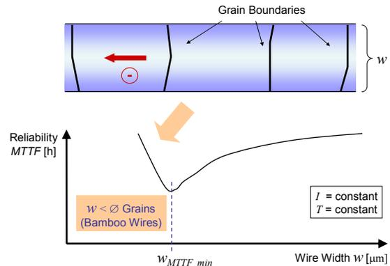
Figure 5. Reduced wire width below the average grain size increases the reliability of the wire with regard to electromigration. So-called bamboo wires are characterized by grain boundaries which lie perpendicular to the direction of the electron wind and thus permit only limited grain boundary diffusion.
