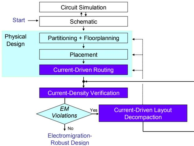
**Figure 11.** Our electromigration-aware analog and mixed-signal design flow includes current-driven routing, verification and decompaction tools intended for an electromigration-robust IC layout.
