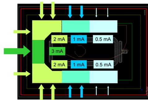
**Figure 9. Current-density correct terminal connections require the verification of all terminal regions with regard to their maximum permissible currents and a subsequent consideration of these values when connecting the wire(s) to the terminal.**
