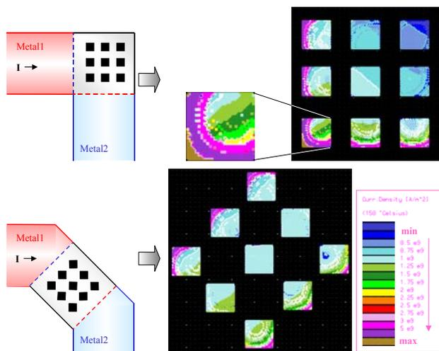
**Figure 7. Current-density distribution within various vias of a via array. In the upper example, the lower and left vias are overloaded while the remaining vias hardly carry any current at all. A better arrangement is presented below.**
