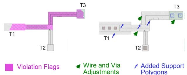
**Figure 14.** Net with current-density violation flags (left) and net and via layout after current-driven layout decomposition (right).
