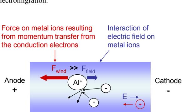
**Figure 2. Two forces are acting on metal ions which make up the lattice of the interconnect material. Electromigration is the result of the dominant force, i.e. the momentum transfer from the electrons which move in the applied electric field.**
