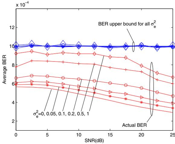
Fig. 6. BER performance of  $2 \times 1$  variable-rate system with the proposed VP-NE strategy and Alamouti code for different estimation error variances.
