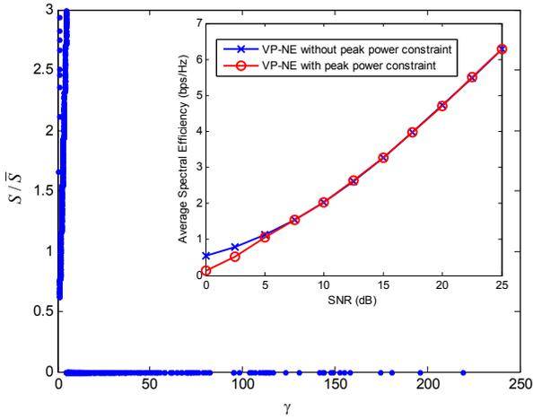
Fig. 9. Normalized temporal power versus  $\gamma^*$  value of  $2 \times 1$  variable-rate system with the proposed VP-NE strategy and Alamouti code, and with peak power constraint:  $S(\tilde{\beta}) \leq 3\bar{S}$ , for SNR=5dB and  $\sigma_e^2 = 0.1$ . In the sub-figure, average spectral efficiency of the VP-NE is plotted versus SNR with/without the peak power constraint.
