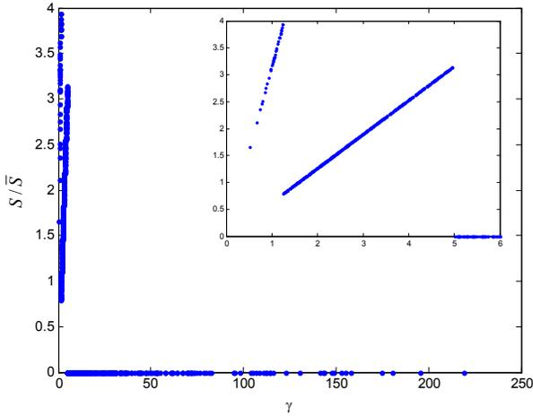
Fig. 8. Normalized temporal power versus  $\gamma^*$  value of  $2 \times 1$  variable-rate system with the proposed VP-NE strategy and Alamouti code for SNR=5dB and  $\sigma_e^2 = 0.1$ .
