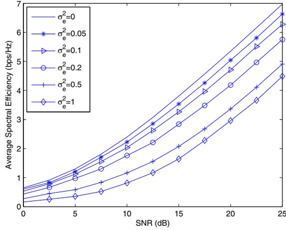
Fig. 5. Average spectral efficiency of  $2 \times 1$  variable-rate system with the proposed VP-NE strategy and Alamouti code for different estimation error variances.
