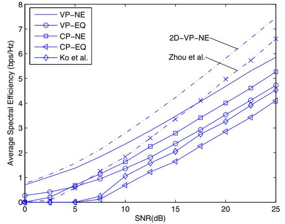
Fig. 4. Average spectral efficiency for  $4 \times 1$  variable-rate system for different power adaptation strategies with  $\sigma_e^2 = 0.2$ . For the solid curves,  $H_4$  code ( $r = 3/4$ ) is used. For the dash curves, the two largest eigen-beams with Alamouti code ( $r = 1$ ) is used for transmission.
