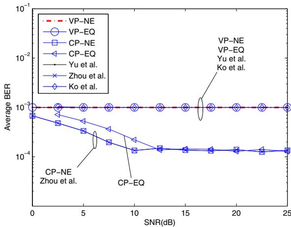
Fig. 3. BER performance of  $2 \times 1$  variable-rate system for different power adaptation strategies with Alamouti code ( $r = 1$ ) and  $\sigma_e^2 = 0$ .
