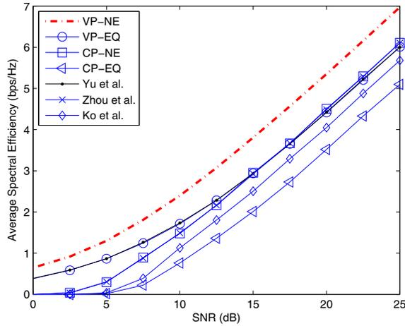
Fig. 2. Average spectral efficiency of  $2 \times 1$  variable-rate system for different power adaptation strategies with Alamouti code ( $r = 1$ ) and  $\sigma_e^2 = 0$ .
