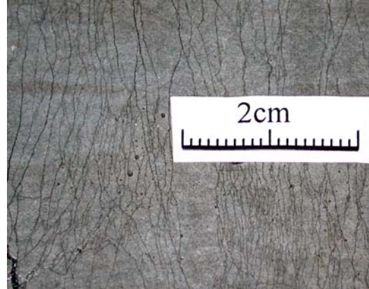
Figure 7: Multiple cracking pattern of PVA-ECC under uniaxial tension
