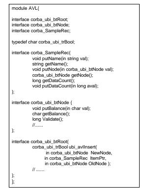
Figure 12: AVL Component Interface Definition
