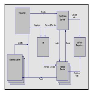
Figure 15: Overall Service Composition Architecture
