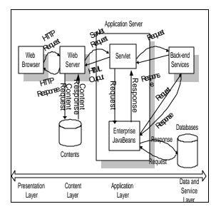
Figure 2: Control Flows in Three-Tier Architecture
