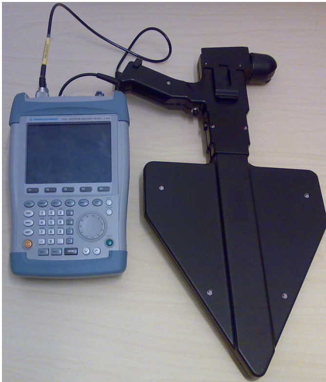
Fig. 4: Rohde & Schwarz FSH6 (model .26) Handheld Spectrum Analyzer [25] with an Empfänger receiver was used in our research laboratory experiments.
