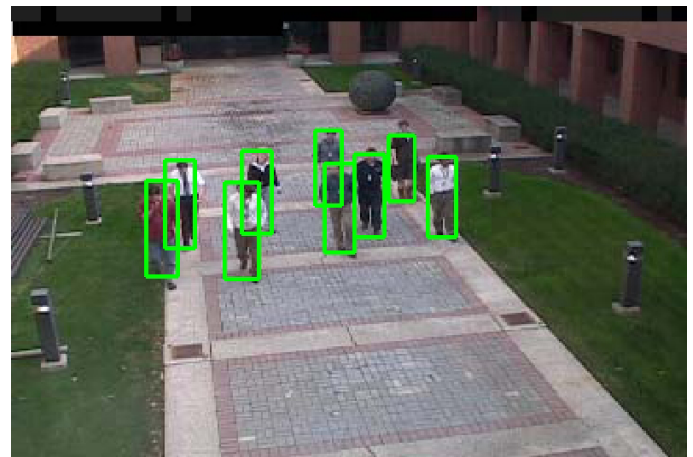
Figure 2. A crowd can be automatically segmented into individuals using on-line global optimization.
