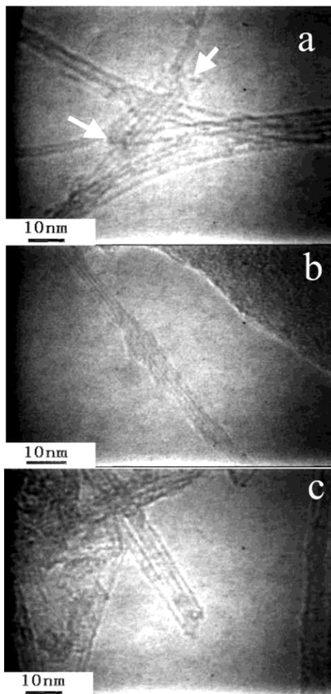
**Figure 9.** Typical TEM images of SWNTs treated with different oxidants: (a) acid mixture (the arrows point to the open ends of tubes); (b) HNO<sub>3</sub>; (c) KMnO<sub>4</sub>.
