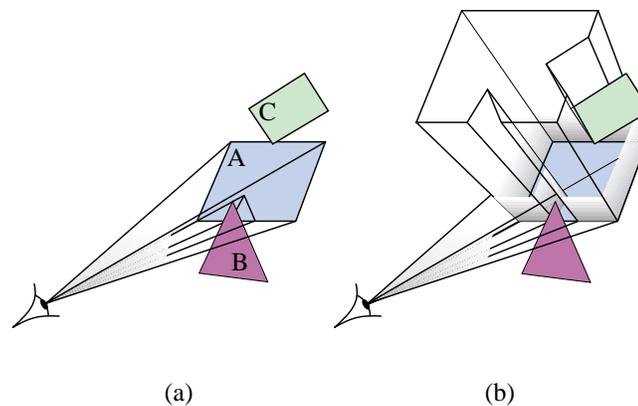
**Figure 5.9:** Beam tracing. (a) A beam is traced from the eye to the scene polygons. It is clipped against the other polygons. (b) Since polygon A is a mirror, a reflected beam is recursively traced and clipped.
