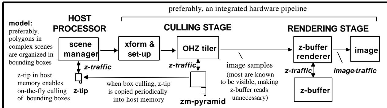
**Figure 1** The proposed architecture for *optimized culling*.
