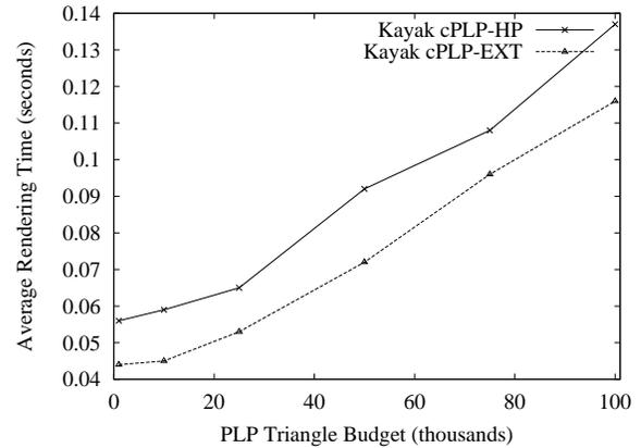
Figure 8: Average rendering times per frame for cPLP-HP and our proposed hardware extension method cPLP-EXT. The PLP budget, reported in thousands of triangles, determines the number of triangles initially rendered to fill-in the depth buffer.
