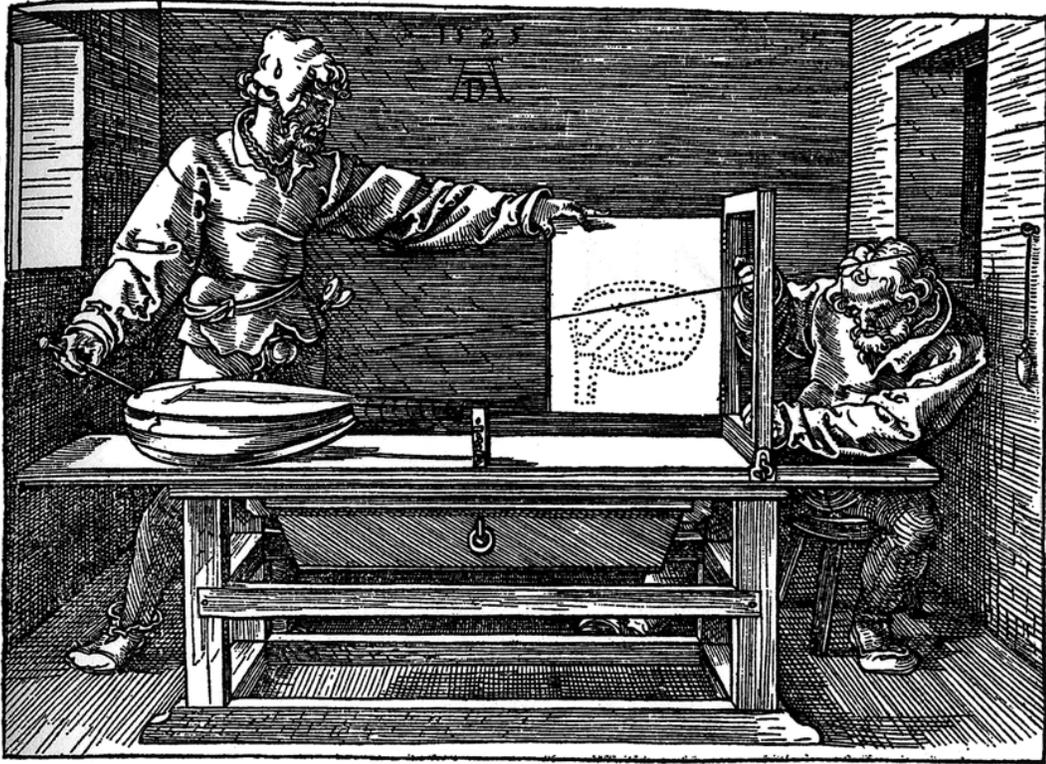
**Figure 4.4:** Drawing by Dürer in 1538 to illustrate his setting to compute perspective. It can be thought of as an ancestor of ray-casting. The artist’s assistant is holding a stick linked to a string fixed at an eyebolt in the wall which represents the viewpoint. He points to part of the object. The position of the string in the frames is marked by the artist using the intersection of two strings fixed to the frame. He then rotates the painting and draws the point.
