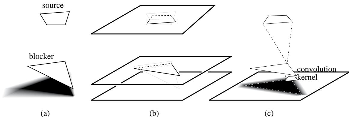
**Figure 6.7:** Soft shadows computation using convolution. (a) Geometry of the scene. (b) Projection on a parallel approximate geometry. (c) The shadow is the convolution of the projection of the blockers with the inverse image of the source.
