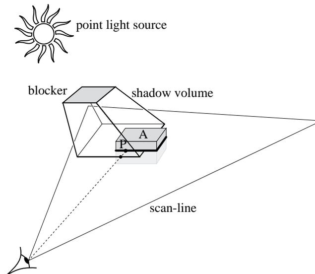
**Figure 5.6:** Shadow volume. As object *A* is scan converted on the current scan-line, the shadowing of each pixel is computed by counting the number of back-facing and front-facing shadow volume polygons on the line joining it to the viewpoint. For point *P*, there is one front-facing intersection, it is thus in shadow.
