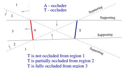
Figure 8: Supporting and separating planes.
