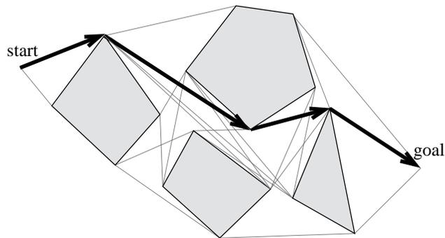
Figure 5.3: Path planning using the visibility graph.
