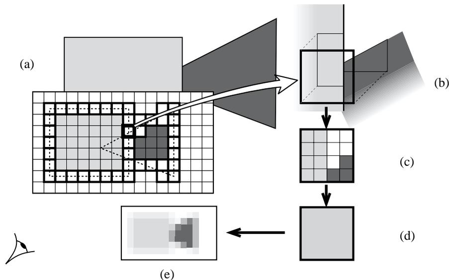
**Figure 4.3:** A buffer. (a) The objects are scan-converted. The projection of the objects is dashed and non-simple pixels are represented in bold. (b) Close-up of a non-simple pixel with the depth sorted fragments (*i.e.*, the polygons clipped to the pixel boundary). (c) The pixel is subsampled. (d) The resulting color is the average of the subsamples. (e) Resulting antialiased image.
