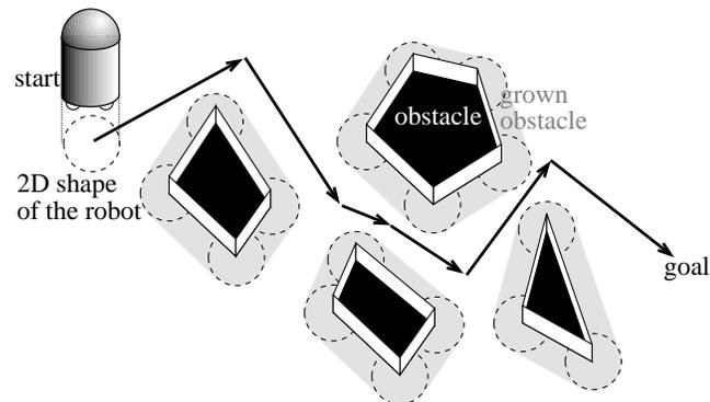
**Figure 2.13:** Motion planning on a floorplan. The obstacles are grown using the Minkovski sum with the shape of the robot. The motion planning of the robot in the non-grown scene resumes to that of its centerpoint in the grown scene.
