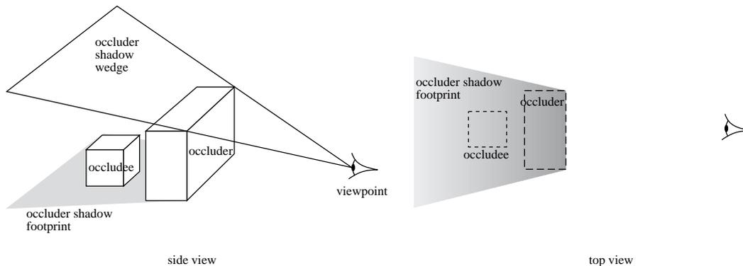
**Figure 6.5:** Occluder shadow footprints. A projection from above is used to detect occlusion. Objects are hidden if they are below the occluder shadows. The footprints (with height) of the occluded regions are rasterized using a z-buffer. Depth is represented as grey levels. Note the gradient in the footprint due to the slope of the wedge.
