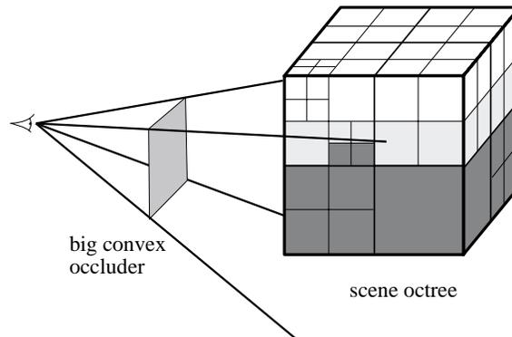
**Figure 5.10:** Occlusion culling with large occluders. The cells of the scene octree are classified against the shadow volumes. In dark grey we show the hidden cells, while those partially occluded are in light grey.
