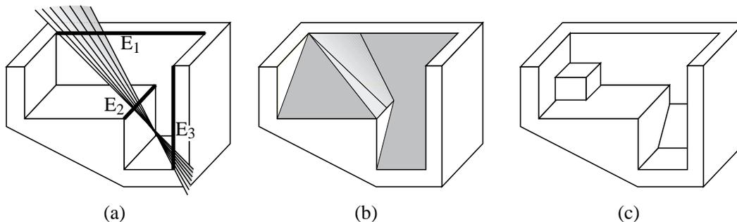
**Figure 5.5:** Visual hull (adapted from [Lau94]). (a) Initial object. A  $EEE$  event is shown. (b) Visual hull of the object (the viewer is not allowed inside the convex hull of the object). It is delimited by polygons and a portion of the ruled quadric of the  $E_1E_2E_3$  event. (c) A different object with the same visual hull. The two objects can not be distinguished from their exterior silhouette and have the same occlusion properties.
