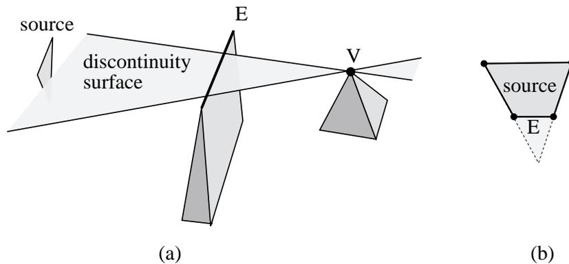
**Figure 7.8:** Complete discontinuity meshing with backprojections. (a) Example of an  $EV$  event intersecting the source. (b) In thick backprojection from  $V$  (structure of the visible part of the source)
