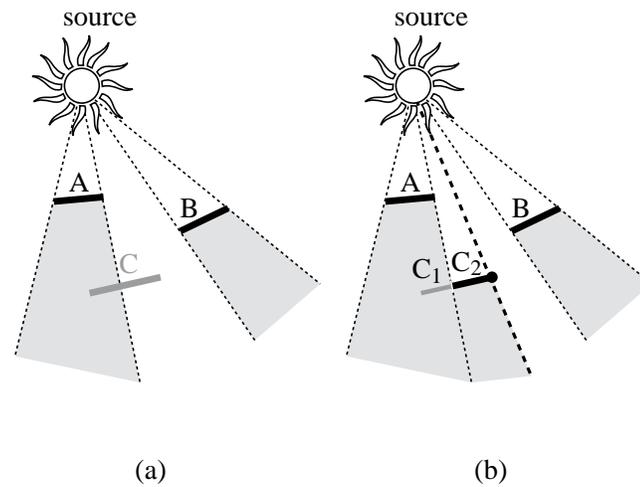
**Figure 5.8:** 2D equivalent of shadow BSP. The splitting planes of the shadow BSP are represented with dashed lines. (a) Polygon C is tested against the current shadow BSP. (b) It is split into a part in shadow  $C_1$  and a lit part  $C_2$ . The boundary of the lit part generates a new splitting plane.
