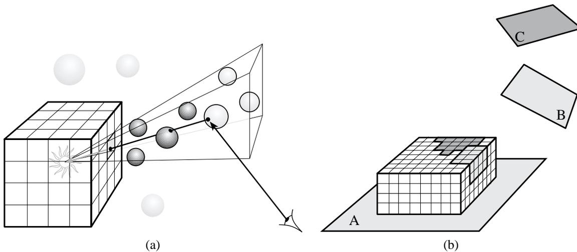
**Figure 6.2:** (a) Light buffer. (b) Form factor computation using the hemicube. Five z-buffers are placed around the center of patch *A*. All form factors between *A* and the other patches are evaluated simultaneously, and occlusion of *C* by *B* is taken into account.
