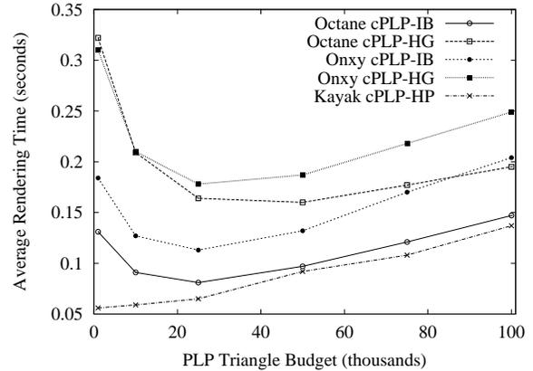
Figure 6: Average rendering times per frame for the implementations of the cPLP algorithm. The PLP budget, reported in thousands of triangles, determines the number of triangles initially rendered to fill-in the depth buffer.
