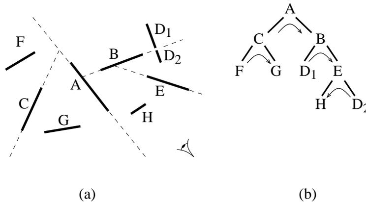
**Figure 5.2:** 2D BSP tree. (a) The scene is recursively subdivided along the polygons. Note that polygon D has to be split. (b) Corresponding binary tree. The traversal order for the viewpoint in (a) is depicted using arrows. The order is thus, from back to front:  $FCGAD_1BHED_2$
