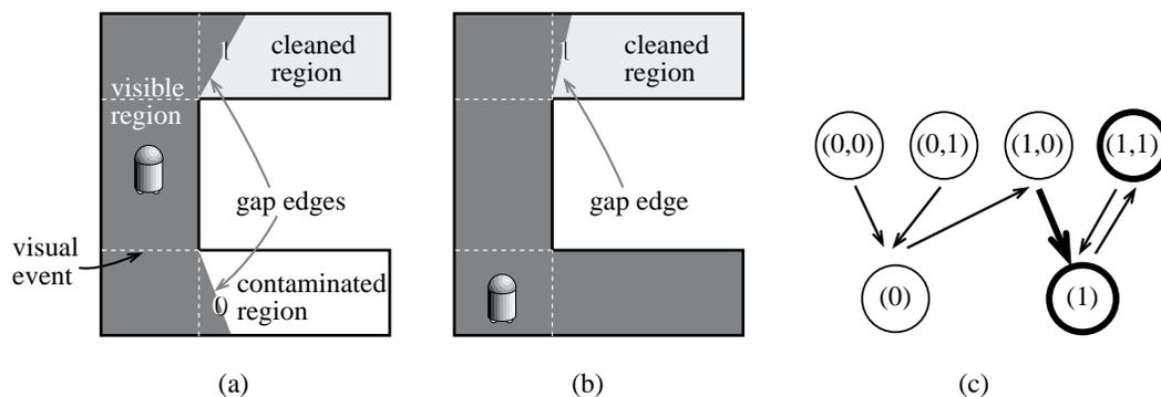
**Figure 7.7:** Pursuit-Evasion strategy. (a) The contaminated region can be cleaned only if the visual event is crossed. The status of the neighbouring regions is coded on the gap edges. (b) The robot has moved to a second cell, cleaning a region. (c) Part of the graph of possible states (upper node correspond to cell in (a) while lower nodes correspond to the cell in (b)). In thick we represent the goal states and the move from (a) to (b).
