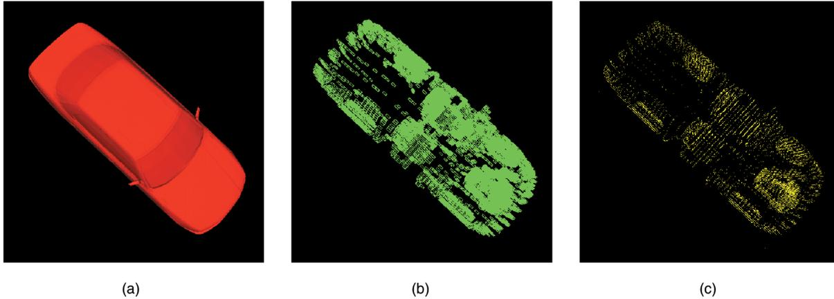
Fig. 3. Occupancy-based spatial tessellation algorithm. The input geometry, a car with an engine composed of over 160K triangles, is shown in (a). Using the vertices of the input geometry, we build an error-bounded octree, shown in (b). The centers of the leaf-nodes of the octree, shown in yellow in (c), are used as the vertices of our Delaunay triangulation.
