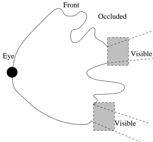
Figure 4: This figure illustrates the technique used in finding the remaining visible cells in cPLP. These cells are found by limiting the remaining work done by the algorithm to only the visible regions.
