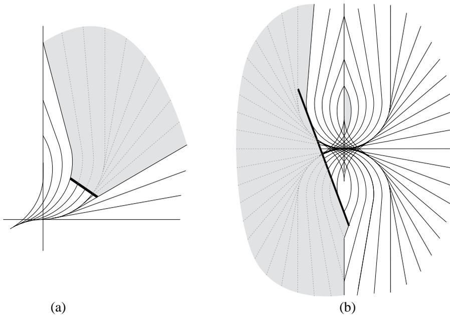
**Figure 5.4:** Shadow for non-holonomic path-planning (adapted from [VLN96]). (a) Simple (yet curved) shadow. (b) Complex shadows. Some parts of the convex blocker do not lie on the shadow boundary. The small disconnected shadow is caused by the impossibility to perform an initial backward circle arc.
