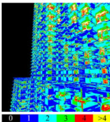
Figure 11. Z-buffer accesses generated by *optimized\_culling* when rendering figure 8 with frame-coherent box culling (1.74 accesses per sample on average).
