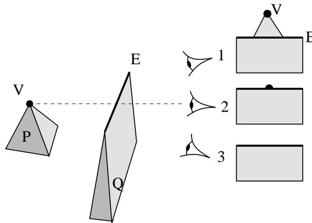
**Figure 3.3:** EV visual event. The views from the three eyepoints are represented on the right. As the eyepoint moves downwards, vertex  $V$  becomes hidden. Viewpoint 2 is the limit eyepoint, it lies on a *visual event*.
