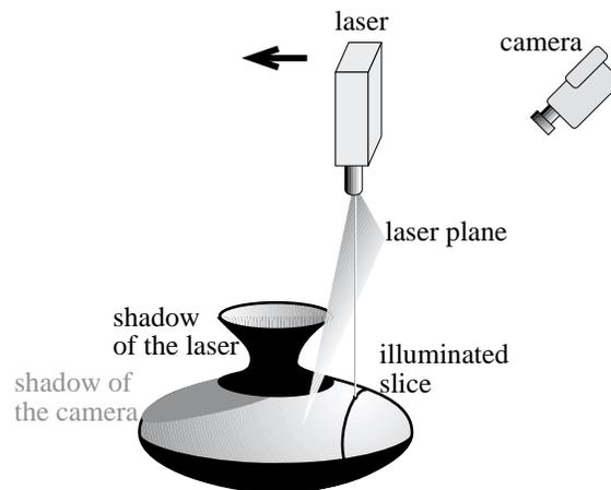
**Figure 2.12:** Object acquisition using a laser plane. The laser emits a plane, and the intersection between this plane and the object is acquired by a camera. The geometry of the slice can then be easily deduced. The laser and camera translate to acquire the whole object. Occlusion with respect to the laser plane (in black) and to the camera (in grey) have to be taken into account.
