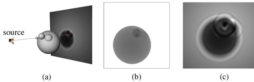
**Figure 6.3:** Non binary visibility for sound propagation. The diffraction by the spheres of the sound emitted by the source causes the diffraction pattern on the plane. (a) Geometry of the scene. (b) z-buffer from the source. (c) Close up of the diffraction pattern of the plane. (Courtesy of Nicolas Tsingos, iMAGIS-GRAVIR).
