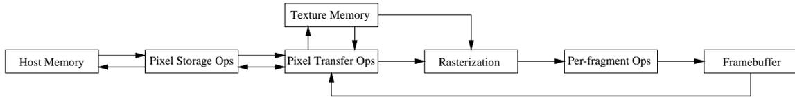
Figure 5: OpenGL imaging pipeline
