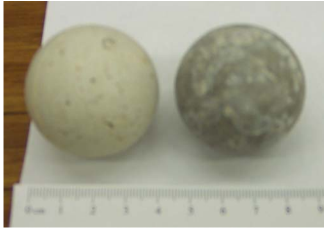
Figure 5.2 An artificial spherical aggregate in (left) and out of the mold (right)
