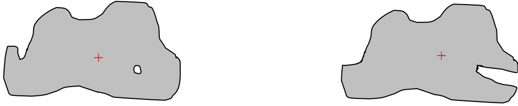
Figure 3.14 A two dimensional particle with overhangs and voids and the virtual particle that will be built using it
