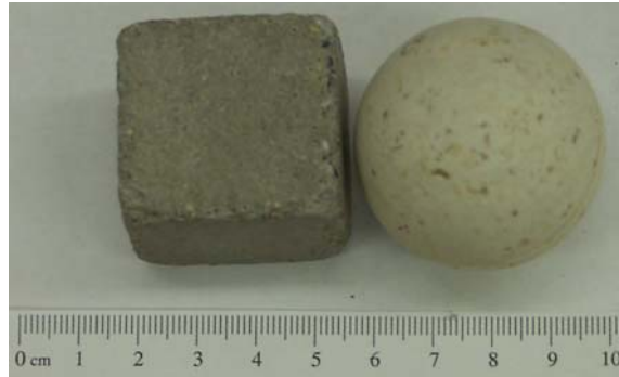
Figure 5.5 The smoothed and roughened surfaces of a sphere and a cube after trial mixtures
