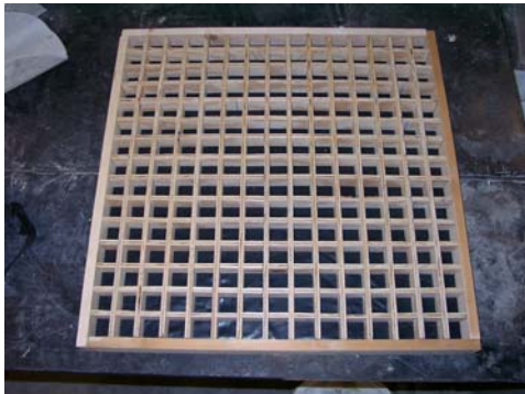
Figure 5.3 The mold used to produce the artificial cube aggregates and a cube ready to be used
