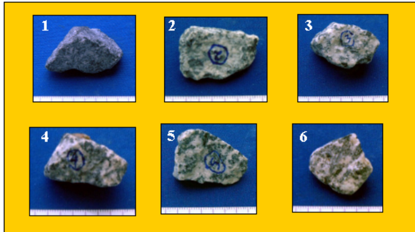
Figure 4.3 The six “WI 0.75” rocks studied from the sieve size range 12.7 mm to 19 mm. The lighter material is feldspar; the darker is hornblende (The smallest division in the scale bars is 1 mm).
