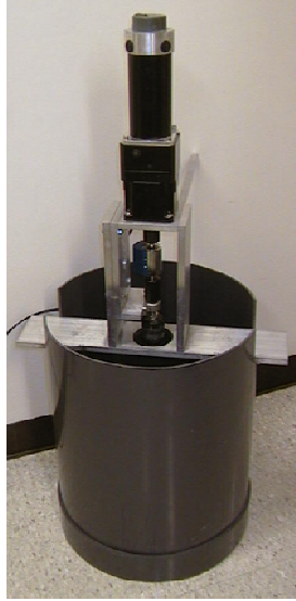
Figure 5.6 ICAR rheometer positioned over its container and the dimensions of the rheometer
