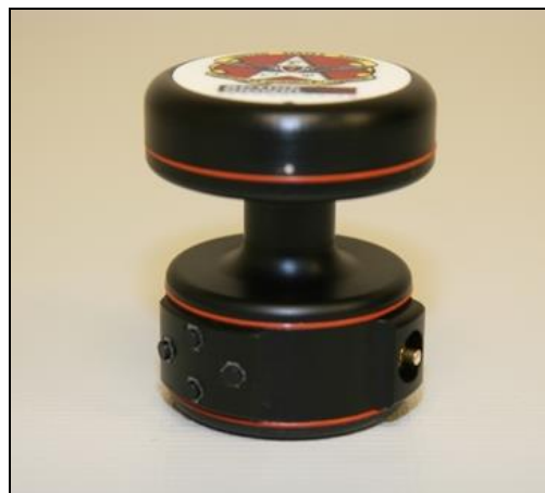
Figure 1: Photograph of the dual-mode, noise-immune stethoscope.
