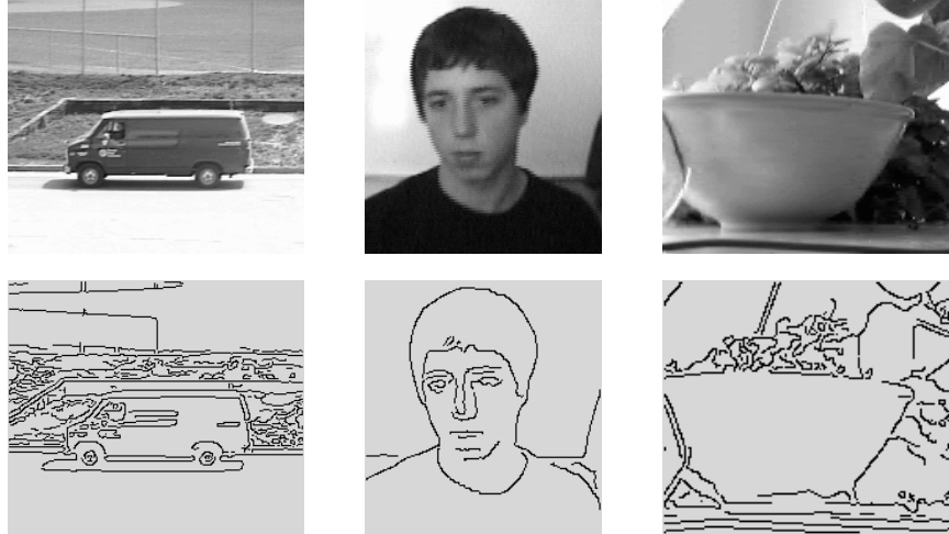
Figure 1: Example of edge detection for shape extraction.
