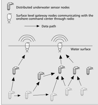
Figure 1. An illustration of the mobile UWSN architecture for long-term non-time-critical aquatic monitoring applications.
