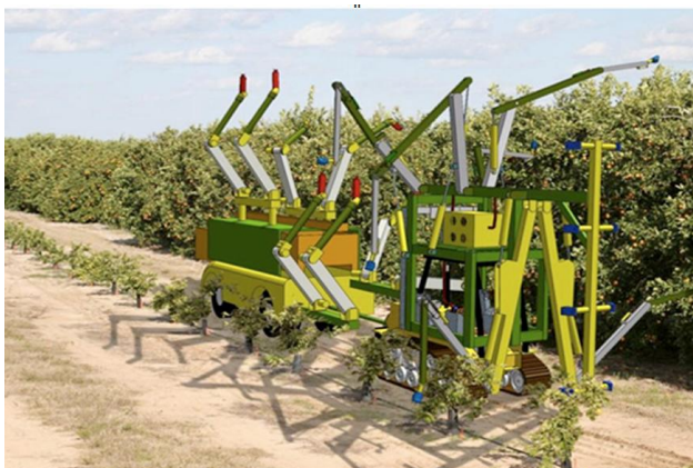
Fig. 4: Robot for picking oranges [14]
