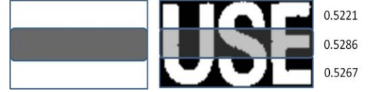
Fig. 16. Stroke distribution estimates by one of the block patterns, and the right values denote the ratio of foreground pixels at corresponding partition regions.
