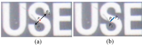
Fig. 15. (a) Probe rays along opposite orientations to search for edge pixels. (b) The two encountered edge pixels P_1 and P_2 are used to estimate the stroke width of character 'S' where feature point P is located.
