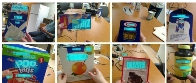
Fig. 23. Example results of localized text regions in cyan from the blind-captured images of text captions.
