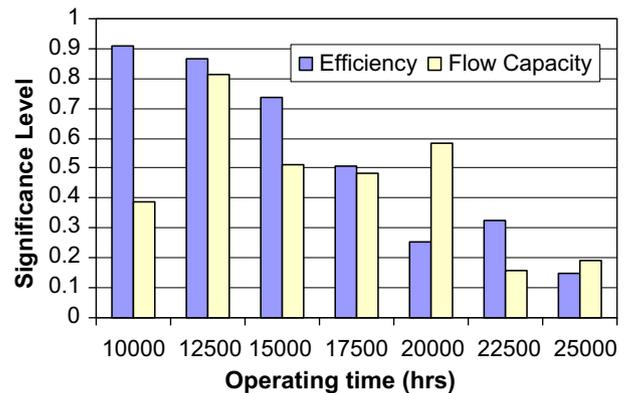
Fig. 12. Significance level of compressor efficiency and flow capacity degradation during engine operation.
