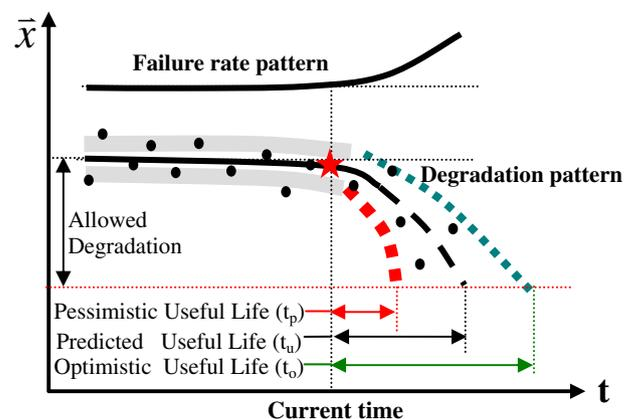
Fig. 1. Degradation and prognostic model.
