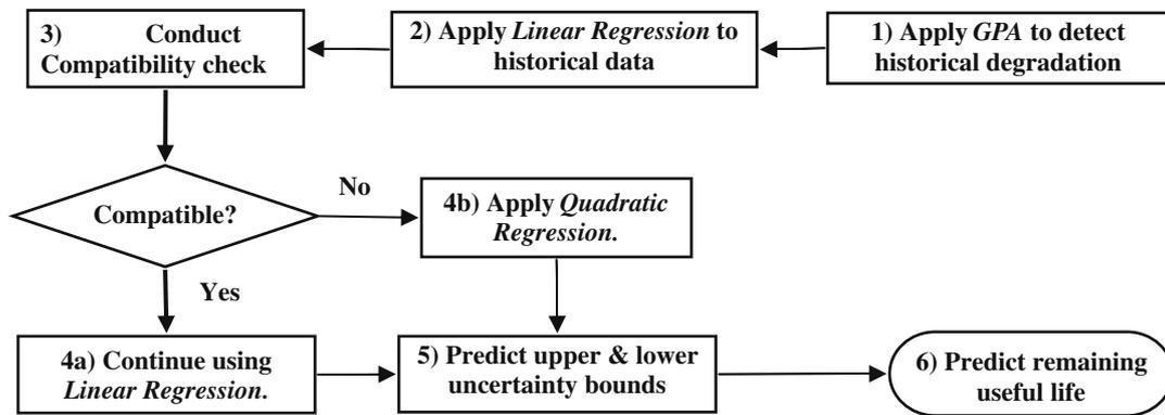
Fig. 6. Diagnostic and prognostics system for gas turbines.
