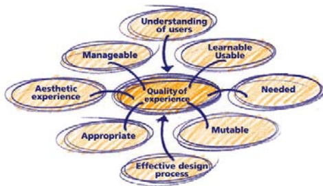
Figure 1: Eight criteria for improving the quality of user experience in the computer interaction design. (Alben 1996)
