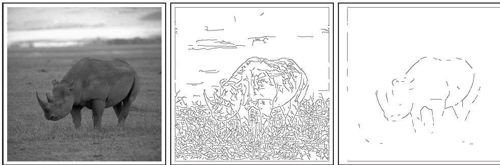
Fig. 1 Edge and contour detection in the spatial domain: The input image (left) is processed by a Gabor energy operator that is motivated by the function of complex cells. The binarized output of that operator is shown in the middle image. The operator essentially acts as an edge detector and does not distinguish the edges that belong to the contour of the animal from those of the background texture. The right image shows the binarized output of a Gabor energy operator that is augmented with surround suppression (Petkov & Westenberg 2003, Grigorescu et al. 2003). The contours of the animal are better visible in this image due to the removal of the texture edges by means of surround inhibition.
