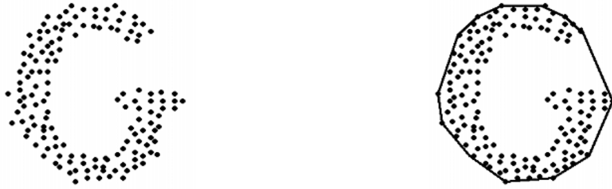
Figure 4.7: Sample images showing a cloud of points(left) and the resultant convex hull(right)
