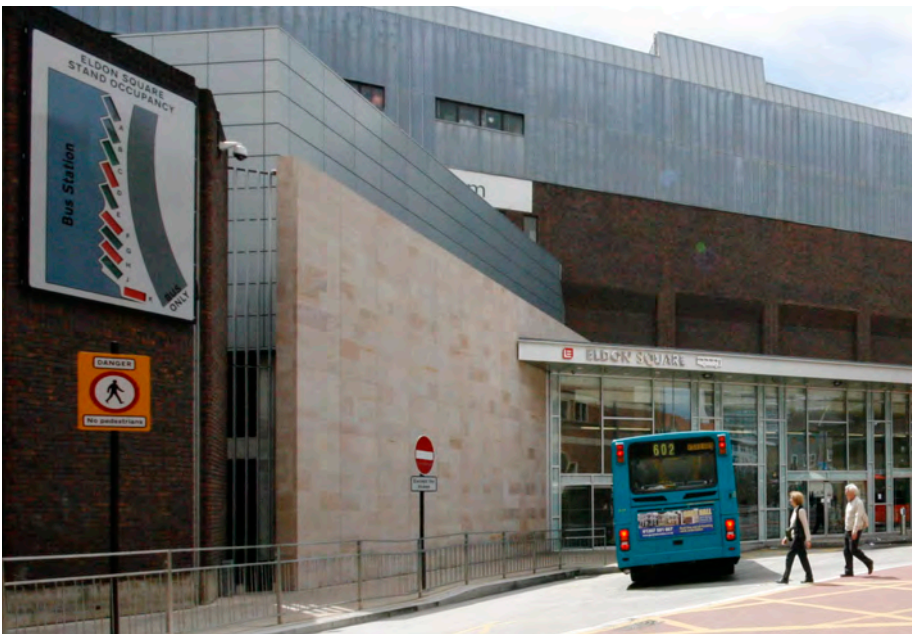
Bay allocation screen advises drivers of the availability of parking bays; layover space is provided to the right for use when bays are occupied.
