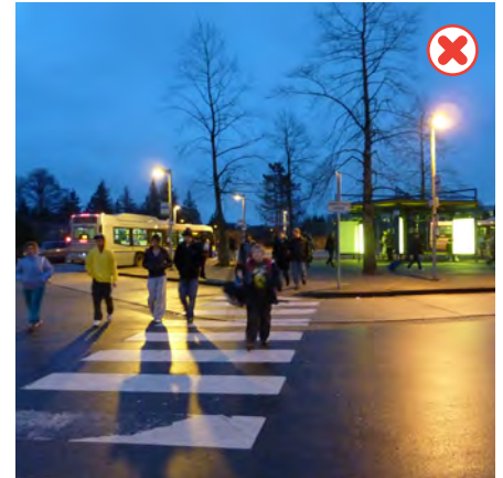
Poor integration with third-party lighting resulting in glare and dark areas. Edmonds Station Bus Exchange, Burnaby.
