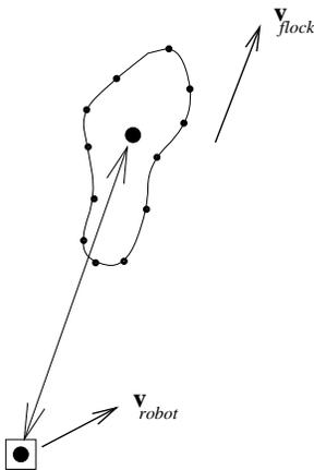
Figure 2: Parameters of the duck tracking system: Robot position and velocity, duck flock shape, position and velocity; separating distance and direction.
