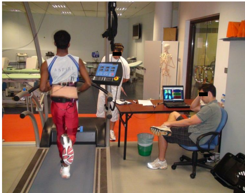
Figure 3.5: Experimental set-up for the studies 2, 3 and 5. Note the X-Pedar data recorder at the back of the runner and the real time recording of the plantar pressure parameter.
