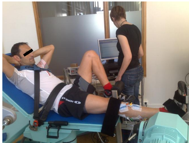
Figure 3.2: Isokinetic testing (study 1) - Positioning of the participant with the knee in extension. Note the position of the electrodes. NB: During the test, the participant held the handles.
