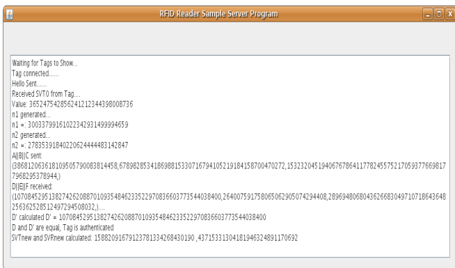
Figure 3. Snapshot of the server-side program executing the RFID reader protocol steps
