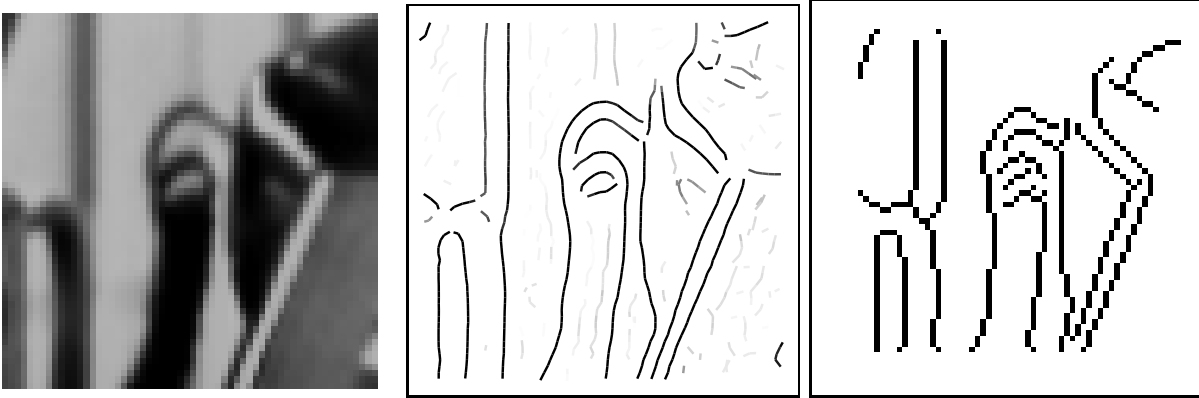
Figure 1: Curve-based representations of image contours computed by the proposed approach (middle) and by more traditional methods (right). The edge representation on the right has been computed by using the Canny’s algorithm implementation of the Matlab’s image processing toolbox.
