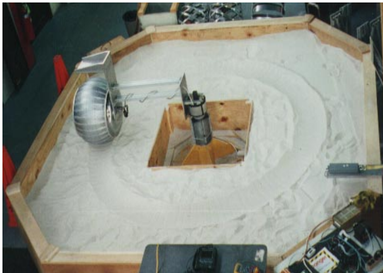
Figure 29: The single wheel testbed was a polygonal sandbox filled with fine grained sand 20 inches deep. The wheel traveled in a 27 foot diameter circle. At the center of the testbed was a slip ring, which provided power and control signals to the wheel. The wheel was supported from the slip ring by two parallel linkages.
