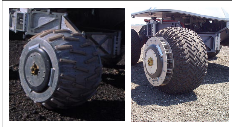
Figure 28: Form comparison of the metal tire with grousers (left) and the pneumatic tire (right).
