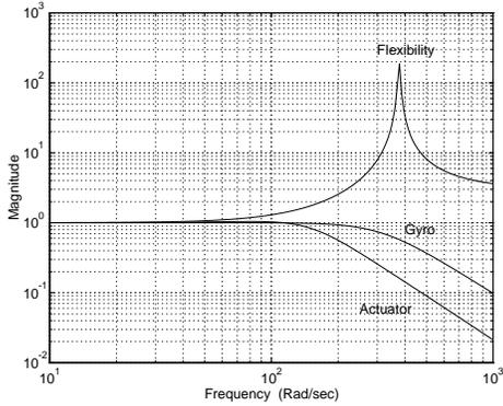
Figure 3: Actuator, Gyro and Flexible Modes Frequency Responses
