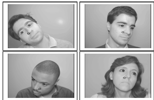
Figure 2: Iris and nose lobe features located by the feature finder in some example test images.
