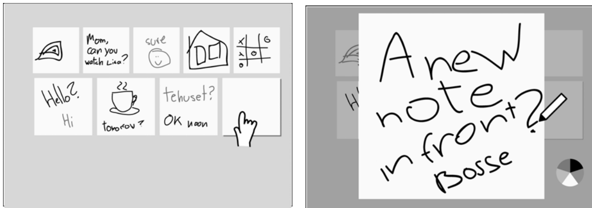
Fig. 3 and 4. Sketches illustrate the two different “views”, which the message board affords. On the left, all notes that have been made are visible. Tapping on the pad in the lower right corner creates a new note. The picture on the right shows a view, where a note is shown bigger in order to afford drawing and writing.
