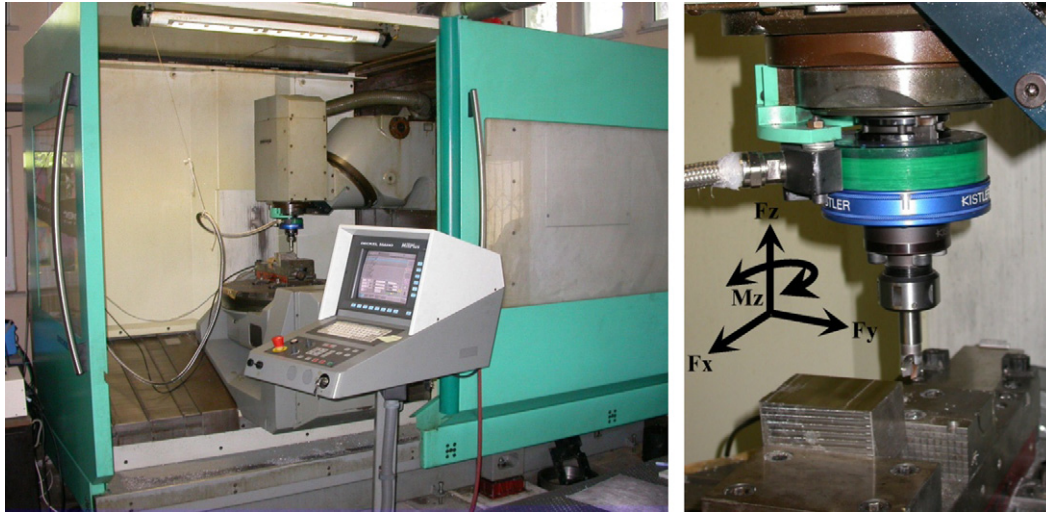
Fig. 1. Experimental setup – machine tool, close-up view of workpiece and RCD setup.
