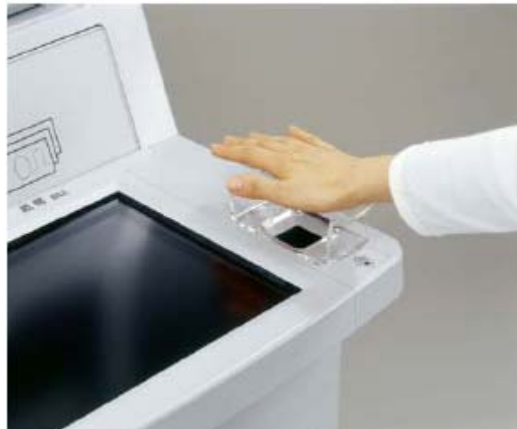
Fig. 6. ATM with palm vein authentication sensor unit
