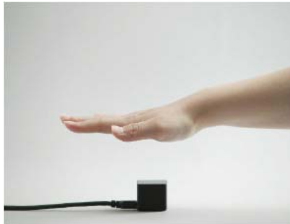
Fig. 3. Contact-less palm vein authentication sensor
