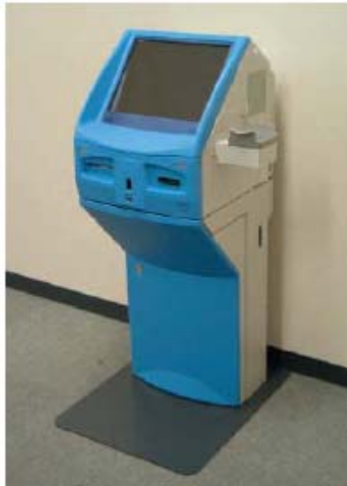
Fig. 7. Information kiosk terminal with palm vein authentication sensor unit
