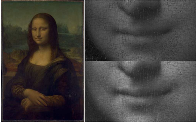
Fig. 4. Left: color composed from multi-spectral data. Right: comparable luminance images made from laser(bottom) and multi-spectral(top) data after registration.
