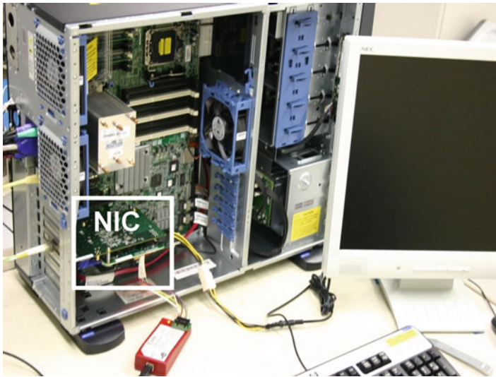
Fig. 15 Target 20 Gbps FPGA-based NIC
