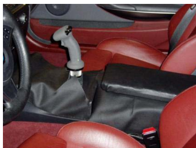
Figure 5. Central console with side stick from Stirling Dynamics Ltd.
