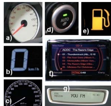
Figure 3. Output modalities: a) analog speedometer b) digital speedometer c) virtual analog speedometer d) indicator lamp e) shaped indicator lamp f) multifunctional display g) digital display
