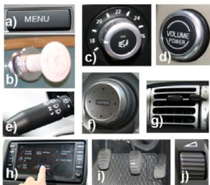
Figure 2. Input modalities: a) button b) button with haptic feedback c) discrete knob d) continuous knob e) stalk control f) multifunctional knobs g) slider h) touchscreen i) pedals j) thumbwheel.
