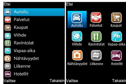
Figure 1. Two alternative menu structures, list and grid, for the driving mode of the navigation software.
