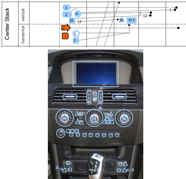
Figure 6. Detailed view of the center stack area. Corresponding markers (vertical) are shown in the photograph.
