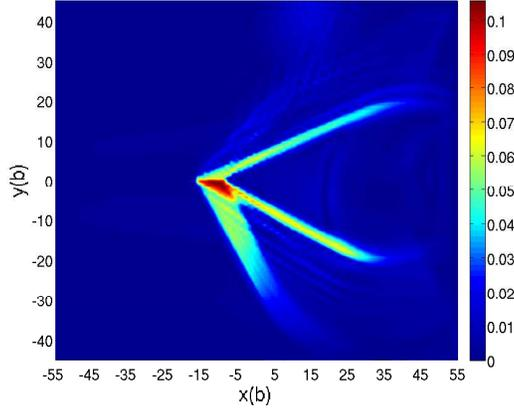
**Figure 46:** Material velocity field around a supersonic dislocation of speed  $2.8V_s$ . The maximum value of material velocity is around  $0.1V_s$ .
