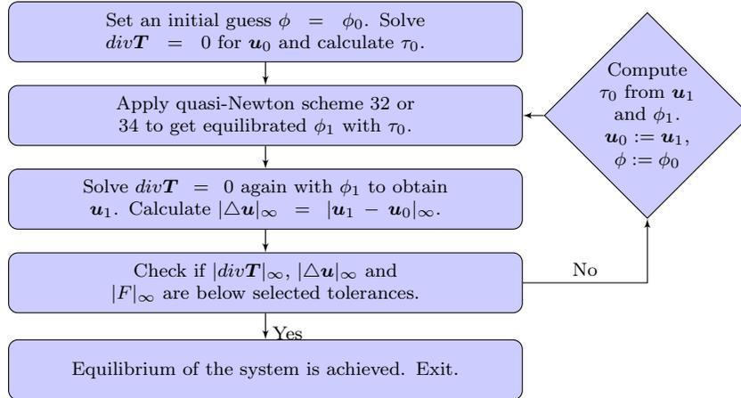
**Figure 4:** Flow chart for equilibrium problems:  $\phi$  and  $\mathbf{u}$  are unknown plastic strain and displacement fields.  $\mathbf{T}$  is Cauchy stress. The initial guess  $\phi_0$  is obtained from a pre-equilibrium solution. Note the repeated initialization of  $\phi$  to  $\phi_0$ , which is found to be crucial for convergence.
