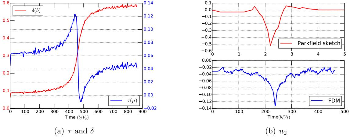
**Figure 54:** Left: layer stress and slip calculated at a fixed point ( $x = -25b$ ) in the passage of a rupture front. Right: transverse displacement at a fixed point in the rupture passage calculated by FDM model compared with sketch of the observed data recorded in the Parkfield earthquake. Sketch adapted from [AR02] (Copyright University Science Books, used with permission).
