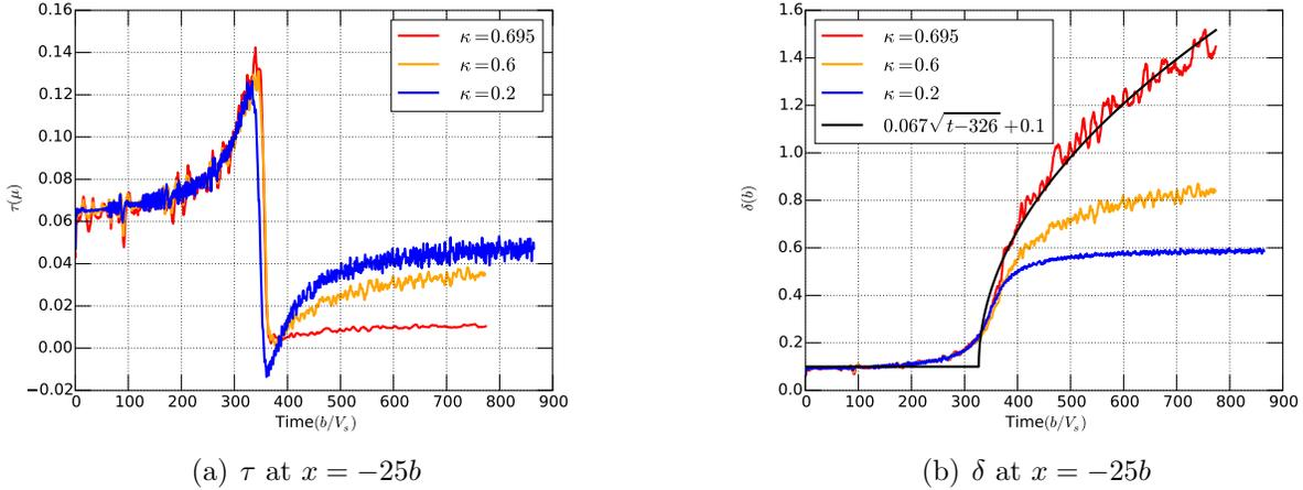
**Figure 55:** Layer stress(left) and slip(right) plotted at a fixed point on rupture front passage with varying elasticity damage.  $\kappa = 0.695$  is fit by a square root function.
