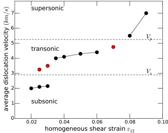
**Figure 42:** Sketch of the MD results from Gumbsch and Gao [GG99], reprinted with permission from AAAS. Dashed lines indicate relevant acoustic wave speeds.
