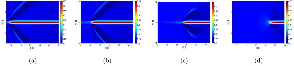
**Figure 51:** *Deformation gradient  $F_{12}$  around shear band.*
