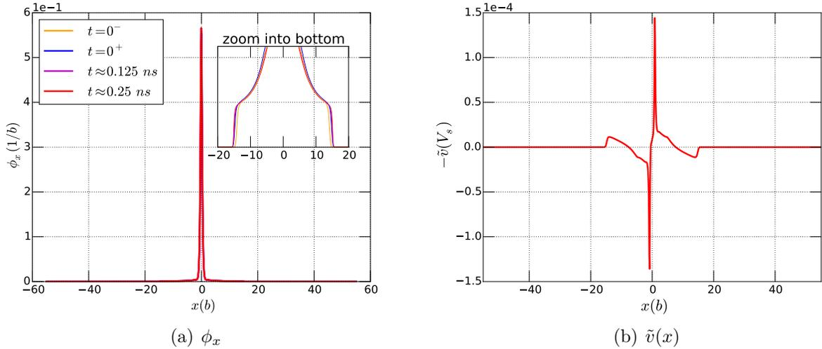
**Figure 18:**  $\phi_x$  and  $\tilde{v}(x)$  of NGB dynamics.  $t = 0^-$  stands for unloaded NGB equilibrium which is used as initial condition. The instant of applying shear load  $5 \times 10^{-5}\mu$  is indicated by  $t = 0^+$ . The dislocation shows no motion but slight shape change at bottom.  $\tilde{v}$  profile persists during the simulation.
