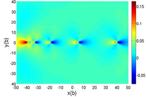
**Figure 16:**  *$T_{12}$  of equilibrated pile-ups under shear load.*
