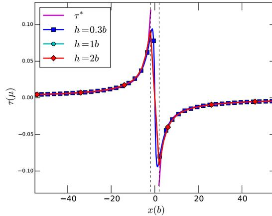
**Figure 6:** Comparison of  $\tau$  with the analytical solution at  $x = 0$ . The dotted lines denote the dislocation core.  $\tau^*$  is a closed-form  $T_{12}$  on  $x_1$  axis from the classic method.  $h$  is the finite element size in the layer, measured with Burgers vector.
