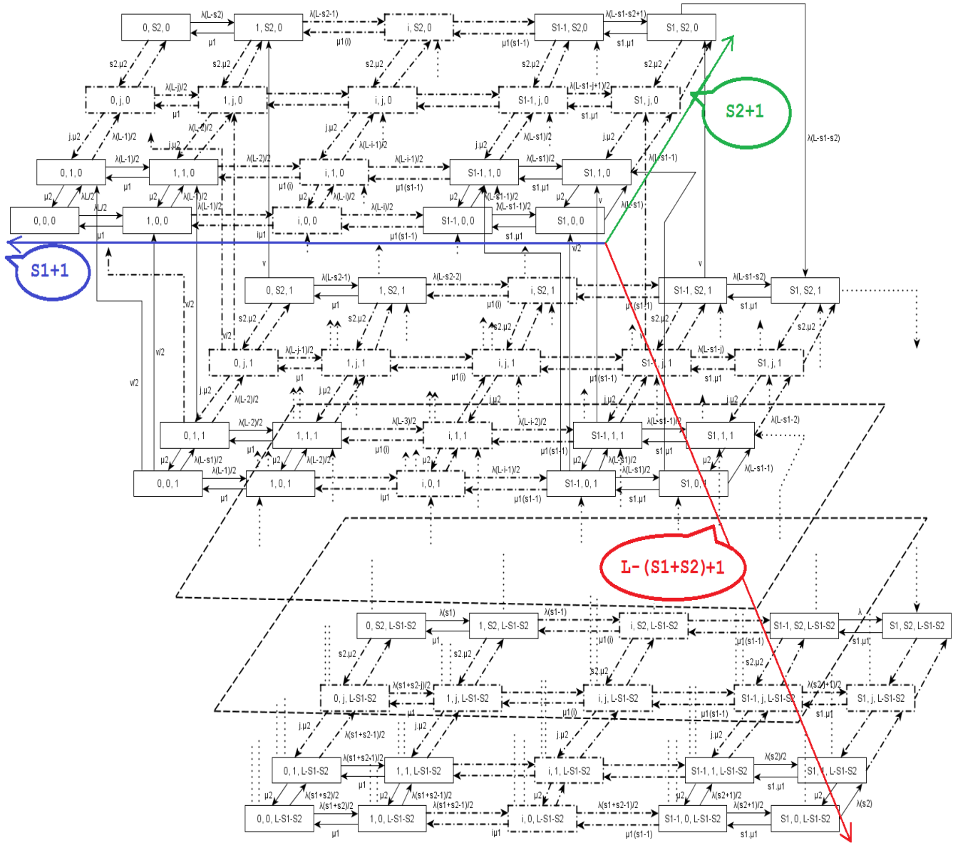
Figure 5. The CTMC describing finite-source retrial networks with two servers classes and Random Server discipline.
