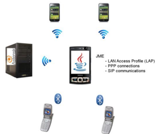
Figure 5. Mobile phone based implementation for community telephone networks.
