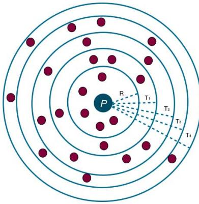
Fig. 1: In the DGT-based proactive localization protocol, each node's concentric data structures (GeoBuckets) are centered on the node itself.
