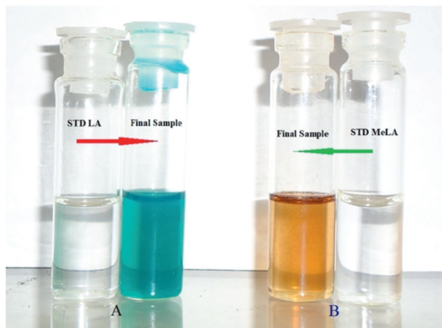
Fig. 8 Final reaction sample of LA hydrogenation in water and methanol (A) final reaction sample of LA in water with Cu–Al 2 O 3 catalyst (B) final reaction sample of MeLA in methanol with Cu–ZrO 2 catalyst. Levulinic acid, 5% (w/w); solvent, water, methanol (95 mL); temp, 473 K; catalyst, 0.5 g; (Cu–Al 2 O 3 , Cu–ZrO 2 ) reaction time, 5 h.
