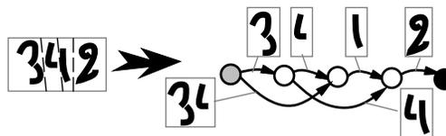
Fig. 16. Building a segmentation graph with Heuristic Over-Segmentation.
