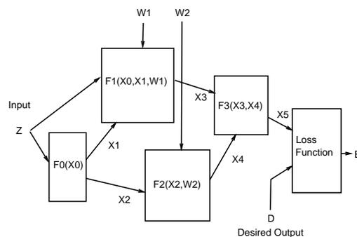
Fig. 14. A trainable system composed of heterogeneous modules.
