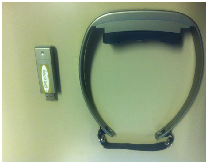
Fig. 2. Outlook of the eeg signal acquisition sensor of brain catcher manufactured by Noroku Kaihatsu Co. Ltd. is used.
