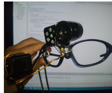
Fig. 3. Proposed glass with two NIR cameras
