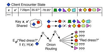
Figure 7: Distributed scheme operation. During an encounter, each peer shares *k* identifiers and an encounter key. Messages are sent using onion routing or an anonymous remailer to preserve anonymity.
