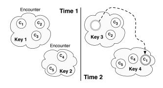
Figure 3: Wireless encounter-key broadcasts provide colocated users with shared state that can later be used to prove participation in an encounter.
