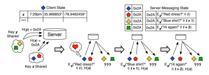
Figure 1: An illustrated sequence of operations. Let H denote a cryptographic hash function and  $E_x(m)$  denote the encryption of message m with key x. Encounter keys x and y hash to the same value, leading the server to relay  $E_x(m)$  to participants in both encounters. However, only participants with key x can recover message m. A timestamp t nonce in the reply prevents replay attacks.
