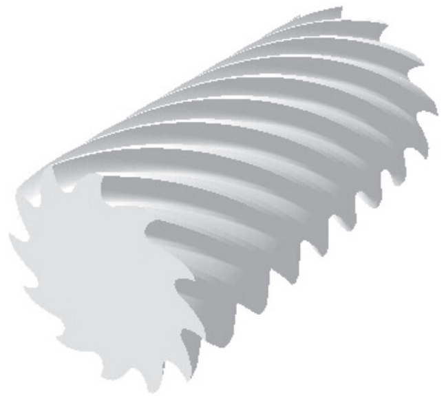
Fig. 9 Solid modelling of the right-hand helical cutting tool
